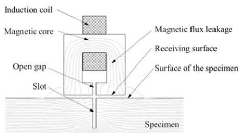
Fig. 2. Principle of magnetic head.
