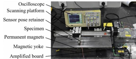
Fig. 12. Experimental platform.
