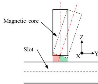
Fig. 4. The head tilted around the X-axis.
