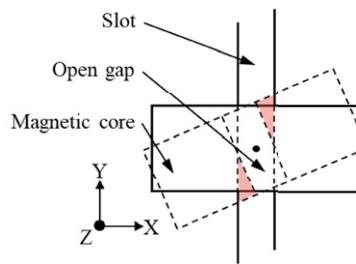
Fig. 8. The head tilted around the Z axis.
