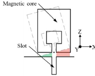
Fig. 6. The head tilted around the  $Y$ -axis.
