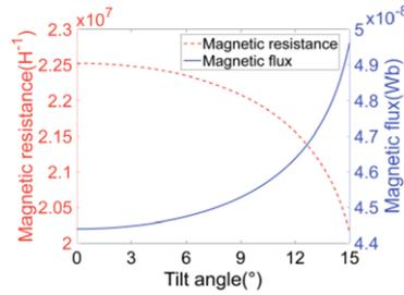
Fig. 7. Relation between air magnetic reluctance/magnetic flux and tilt angle.
