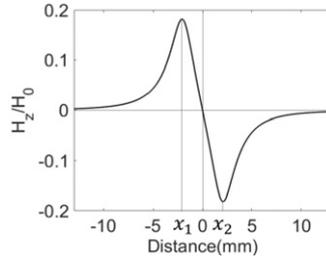
Fig. 9. Distribution of the vertical component of the leakage magnetic field.
