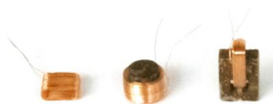
Fig. 1. Single coil, iron-core coil and magnetic head.
