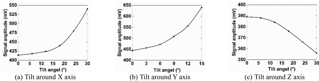
Fig. 14. Experimental results of the influence of tilt around different directions on detection ability.
