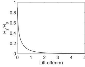
Fig. 5. Relationship between vertical component of leakage magnetic field and lift-off.
