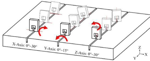
Fig. 3. Heads are tilted around three directions: X, Y and Z.
