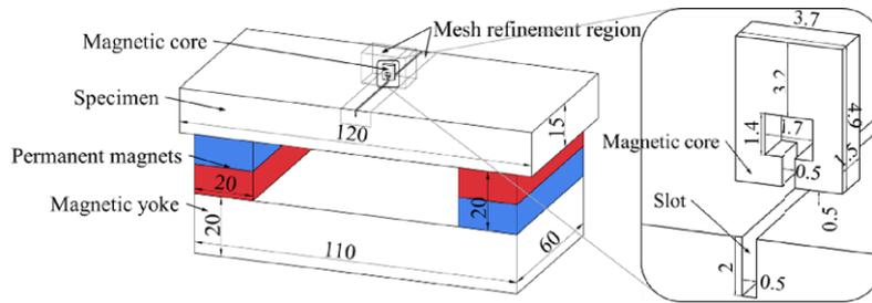
Fig. 10. Simulation model.
